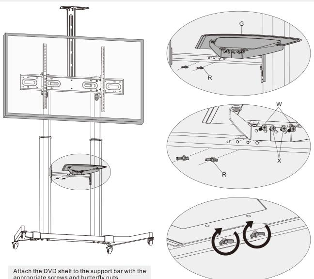
Attach the DVD shelf to the support bar with the appropriate screws and butterfly nuts.
