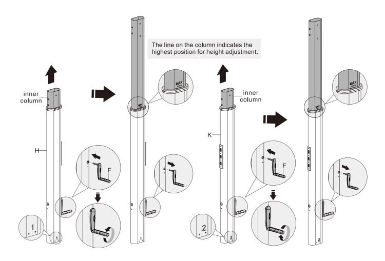
Attach the handle to the column marked with "1".
