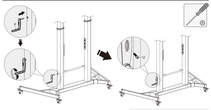
Use the handle to adjust the columns to the desired height and secure using the appropriate screw.
