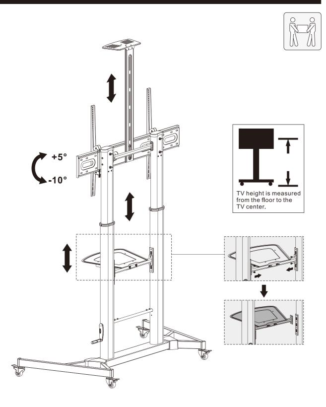
**Note:** It is recommended to adjust the columns to the desired height before installing the display.
