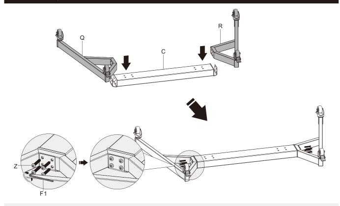
Attach the right base to the middle base and secure with screws(Z). Repeat this step for the left base.
